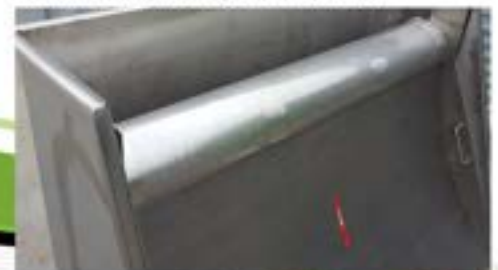
Stainless steel wedge wire screen.
